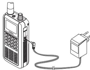
If rechargeable batteries are installed and **ALKALINE/Ni-MH** is set to **NI-MH**, the adapter powers the scanner and recharges the installed batteries at the same time.
