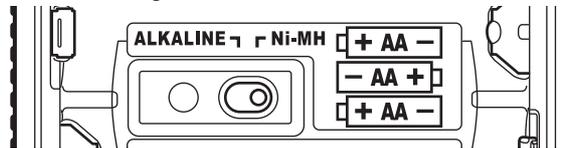
1. Remove the battery cover and set the battery switch.
